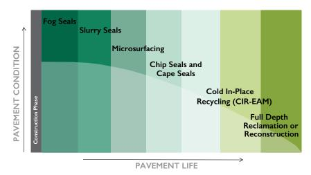
Because of the high strengths available with foamed asphalt, it can be cost effectively applied earlier in a pavement's life, helping maintain high levels of serviceability.
